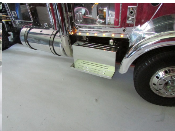
Install step mounts upside down for Cab to Step Clearance
