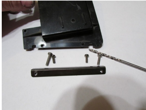
Drill out self tapping holes to # 30 drill bit
